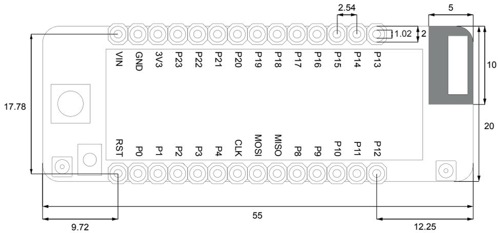
Figure 5 – Mechanical drawing (top down view) – Units: mm
