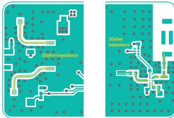
Figure 7 – 50-ohm impedance antenna connections
