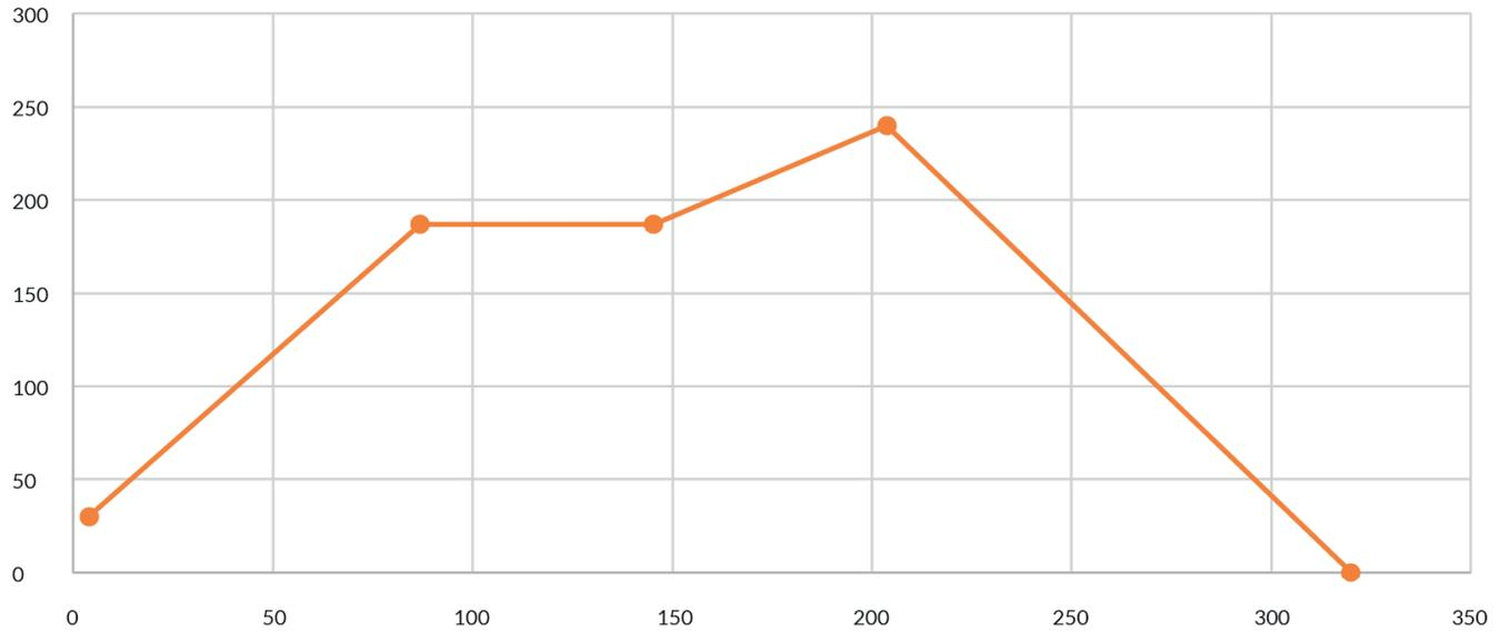
Figure 10 – Reflow soldering temperature profile
