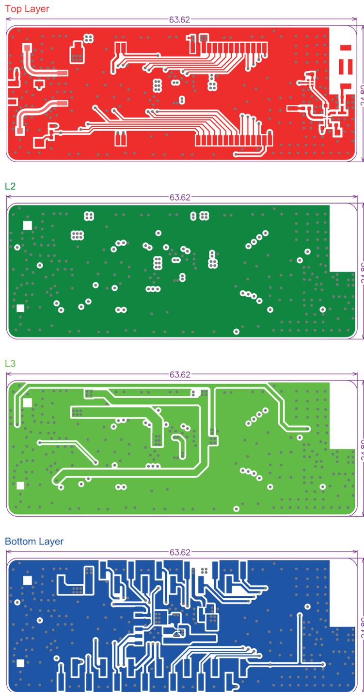
Figure 9 – PCB layers for reference design – Units: mm
