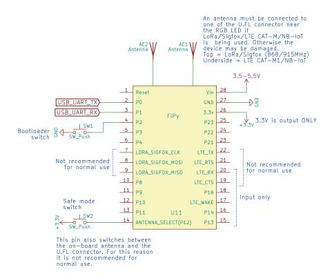
Figure 3 - Minimum required circuit
